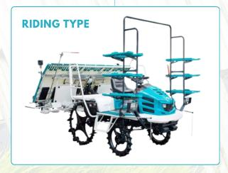
All over the world, a riding-type rice transplanter operates similarly to a walk-behind model, but it is often faster and has a larger capacity. Because of its speed, it must be controlled like a vehicle. This type can plant additional rows of rice seedlings, making it an ideal choice for larger rice fields.
